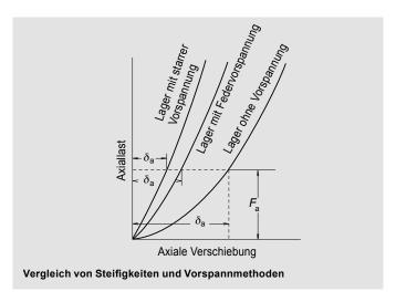
$$F_{\text{a min}} = \frac{C_{0\text{a}}}{100} \cdot \left(\frac{n}{N_{\text{max}}}\right)^2$$
