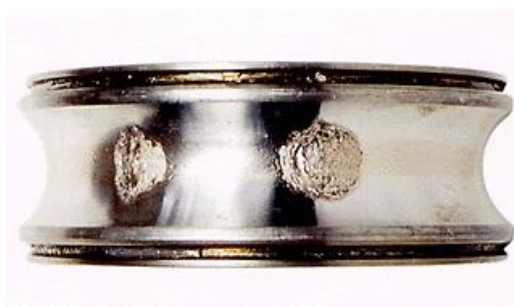
Fig.3 Appearance of spalling 1)
